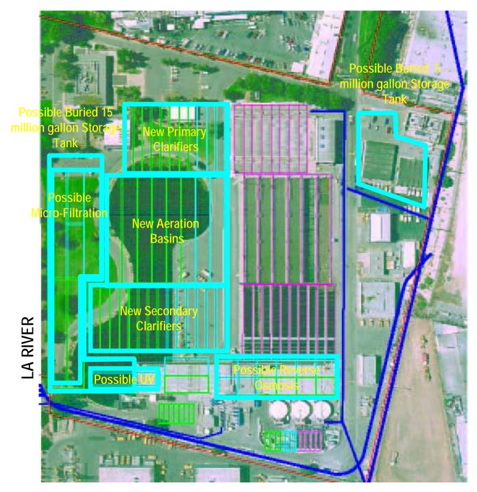
Figure 8-8 Los Angeles-Glendale Water Reclamation Plant Options: Ultimate Site Buildout Plan with Added Storage
