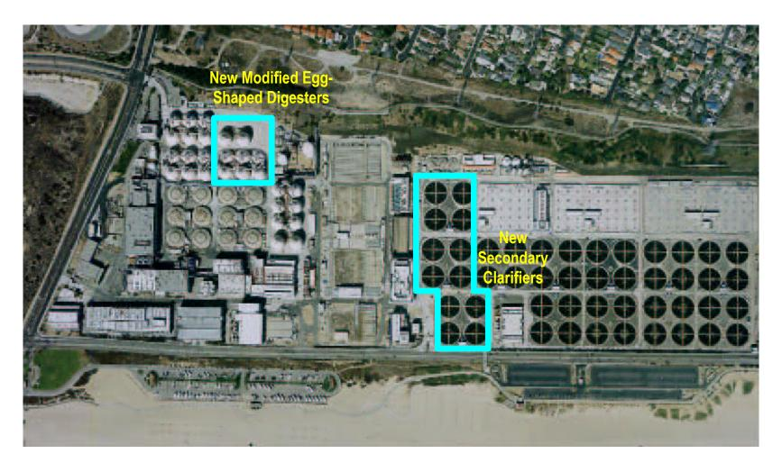
Figure 8-5 Hyperion Treatment Plant Options: Expansion to 550 mgd
