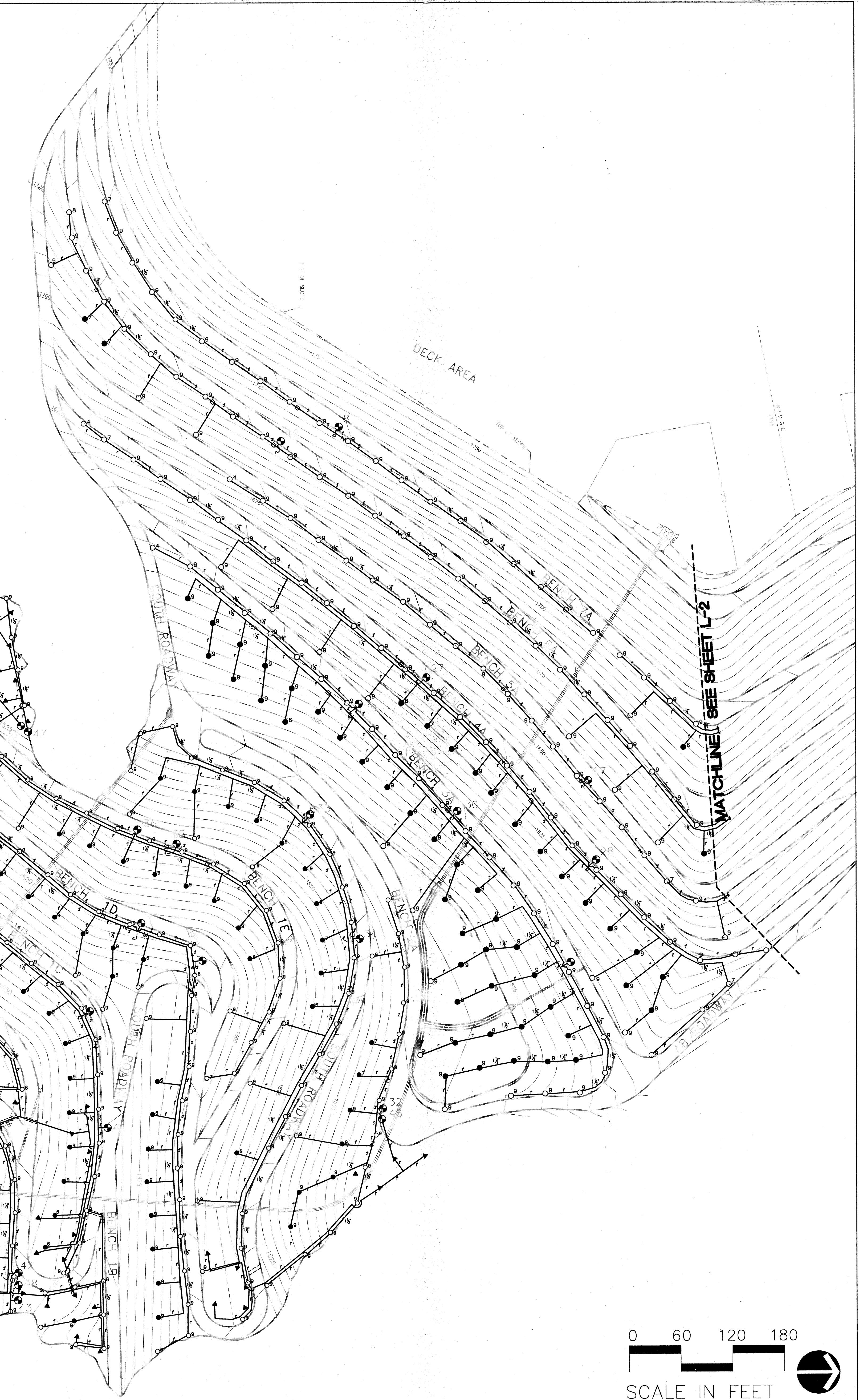
IRRIGATION HEAD &amp; LATERAL LINE PLAN
