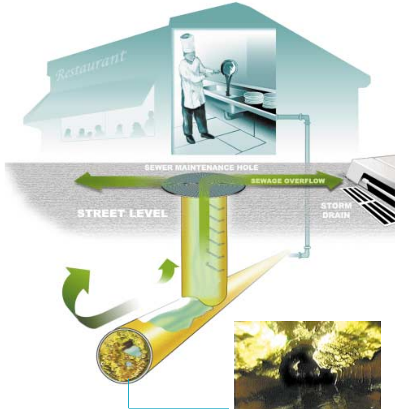
Actual photo taken by remote controlled camera showing grease buildup in sewer pipe interior.
