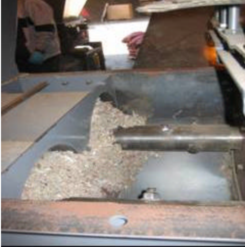
Feedstock in auger mixer
