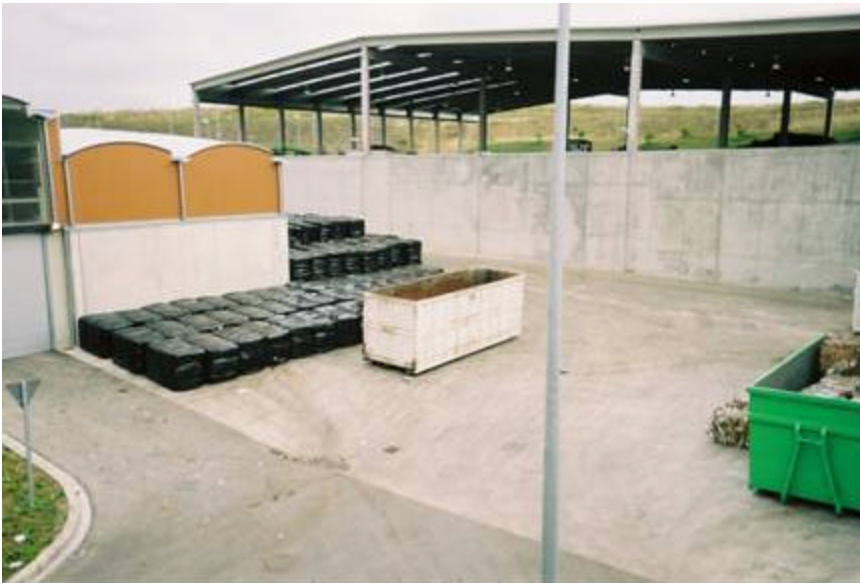
Wrapped reject bales ready for the landfill; unwrapped bales to the right
