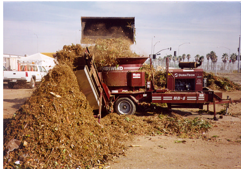
City Yard Trimmings-Grinder Operation
